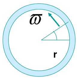
$\omega$  Is angular velocity of ring
