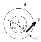
The acceleration is produced by the vector sum of the two forces, which in this case is directed inwards and has magnitude  $\frac{V^2}{R}$ , where V is the windspeed and R is the distance to the centre of the cyclone.
