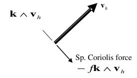
opposite sign in the southern hemisphere, the sense of the specific Coriolis force is directed to the left of the wind in that hemisphere.
