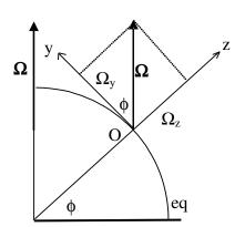
is to treat the earth as locally flat. That is, we consider that the earth's surface in the vicinity of a point stays close to the tangent plane. Take a position O on the surface of the Earth. Then we shall take rectangular co-ordinates Oxyz such that Oxy is the plane which is tangential to the Earth's surface at O, with Ox directed eastward, Oy to the North and Oz directed vertically upwards at O. That can, of
