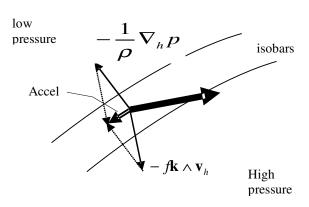
specific pressure gradient force is perpendicular to the isobars. The nett resultant of these two forces produces the acceleration, shown in the sketch as the open arrow.
