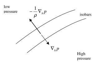
Putting these forces together (and recalling that we are only discussing horizontal components here) we get the situation shown to the right. The direction of the isobars (thin curves) and the direction of the wind (broad arrow) have been arbitrarily chosen. The specific Coriolis force is perpendicular to the wind and the
