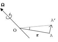
In the sketch  $\Omega$  is the rate of rotation vector of the rotating frame relative to the fixed frame. It is defined to be pointing along the axis of rotation in the sense of a right-handed corkscrew. The rate of angular rotation is  $|\Omega|$ .
