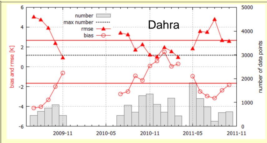
The land cover at Dahra, Senegal, is tiger bush with a TCC of 4%. The long data gap from Dec 2009 to Jun 2010 is due to theft of solar panels. Due to its sub-tropical climate, Dahra has the fewest data points of the four stations (many cloudy satellite pixels).
